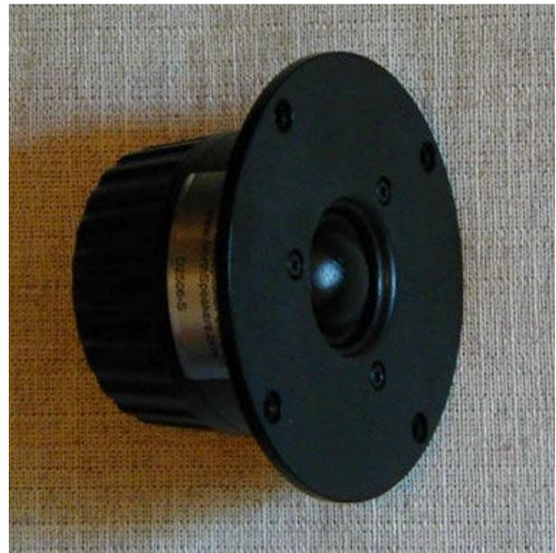
Most chambered dome tweeters employ a very soft half roll surround to allow the lowest resonance frequency. A 25mm dome with a half-roll suspension can still achieve a fundamental mechanical resonance of only a few
